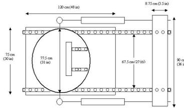
FIGURE 6. The Linear Pendulum Apparatus
