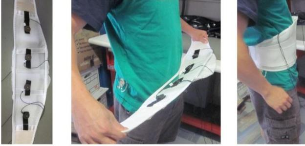
Figure 3: Belt with four C2 tactors, and placement of vibrotactile belt on user.
